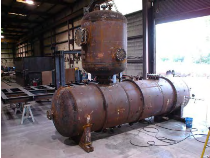
Deaerator tray tank and storage tank during Hydrotest.
