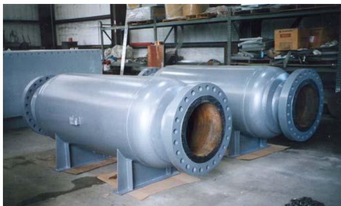
Inline Silencers after Hydrostatic test
