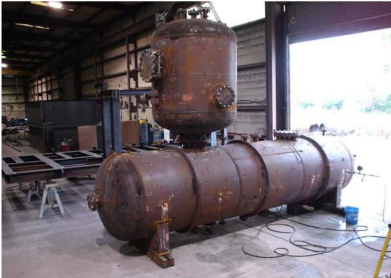
Deaerator tray tank and storage tank during Hydrotest
