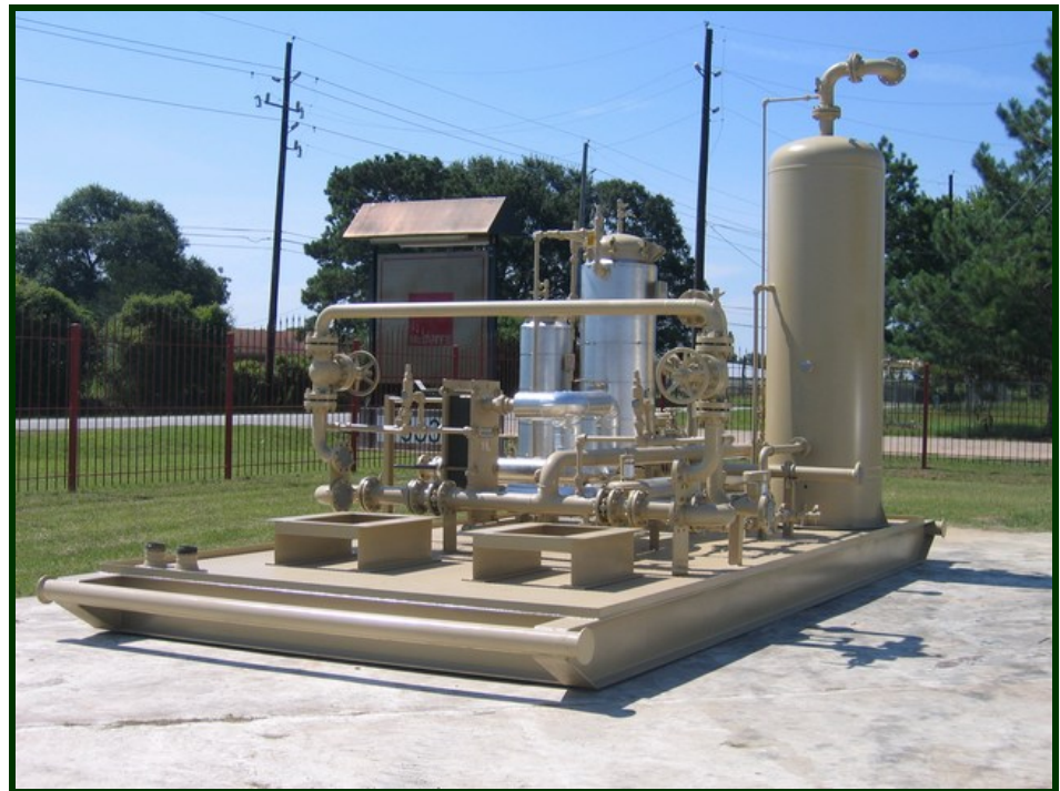
Regeneration Skid prepared for shipment
