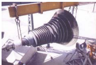
GE 540 MW Steam Low Pressure Rotor
