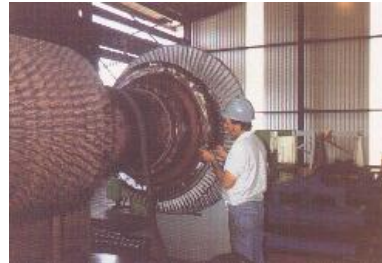
GE Frame 5 Combustion Turbine Bucket Replacement
